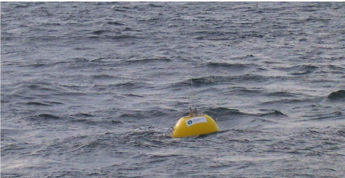
**Photo 1:** Deployed directional Waverider buoy (Photo: Environment Agency)
