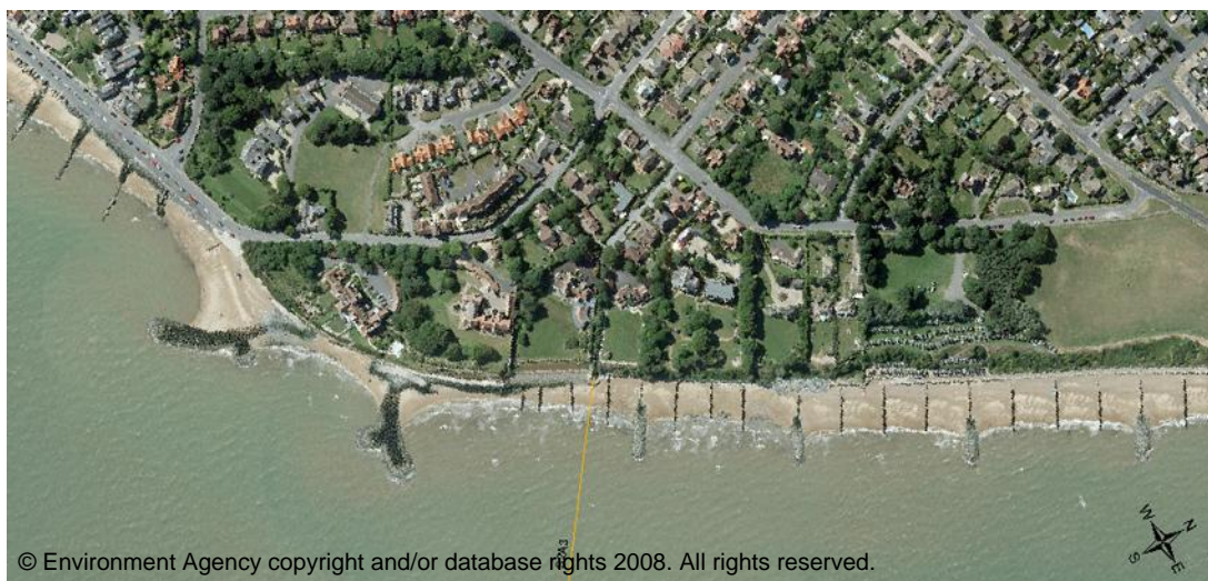
Photo 3: Rock groynes along the Felixstowe frontage in 2008 (location of EA survey transect S2A3). (Photo: Environment Agency)
