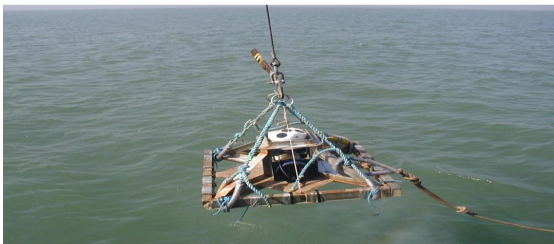
Photo 1: AWAC in frame being deployed (photo: Gardline Environmental) (Photo: Environment Agency)
