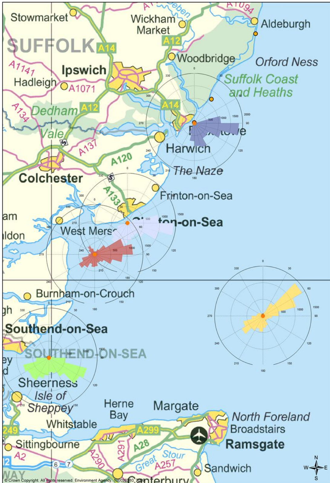
Figure 7: Main wave coming direction (Mdir) and occurrences for the Essex AWACs and the offshore waverider buoy, from October 2007 to September 2008.
