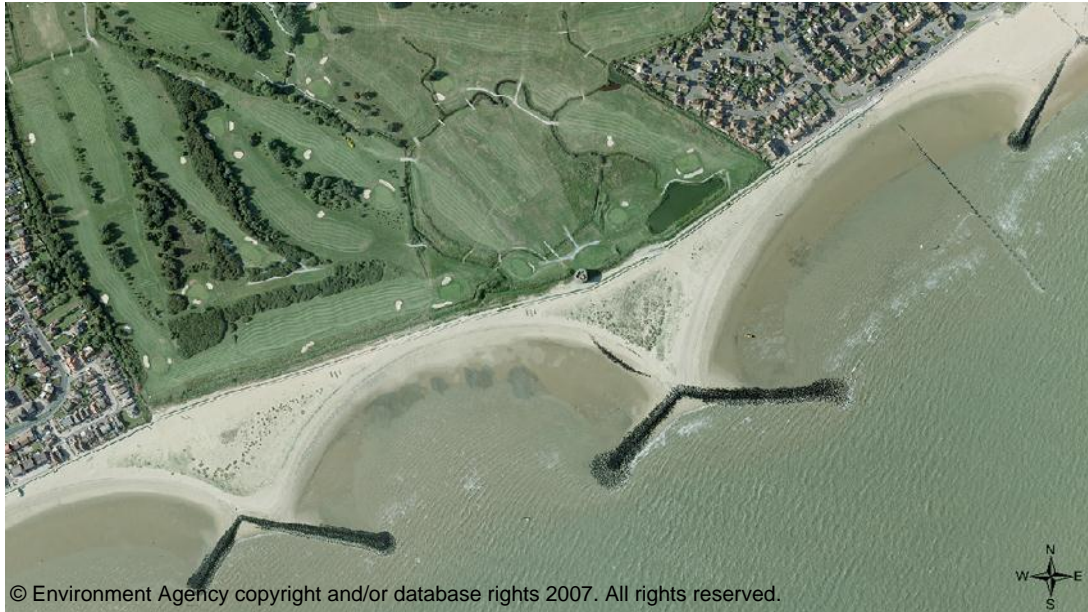
Photo 5: Aerial photograph of the sandy beach and fish tail groyne in front of Clacton golf course in 2008 (location of EA survey transect E1A7).
