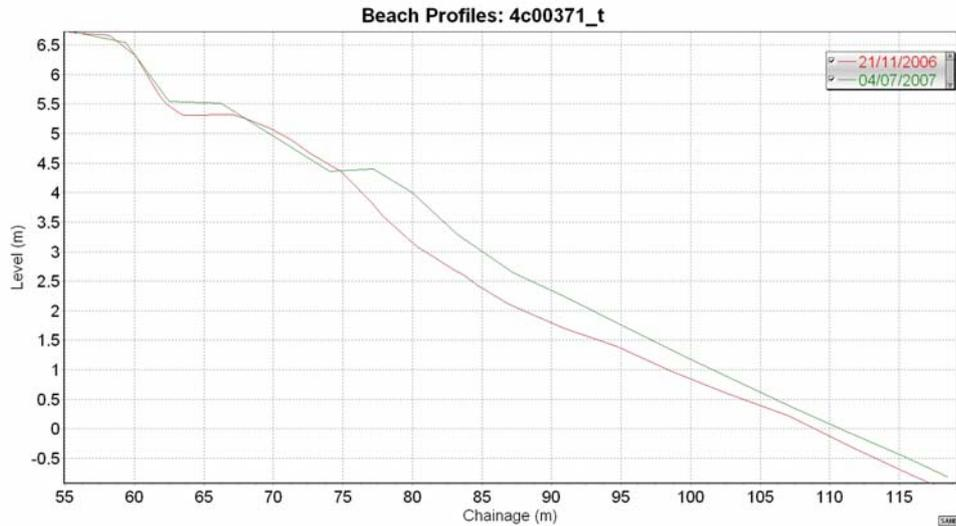
Figure 3.6-1: Example of improved crest width
