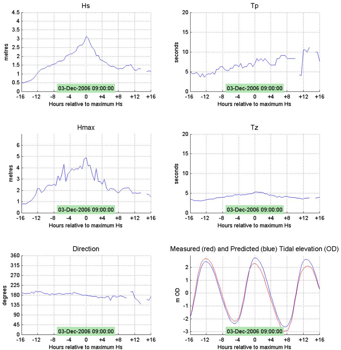
Figure 3.100-1: Example of wave statistics for 03<sup>rd</sup> December 2006 storm
