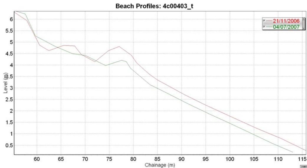
**Figure 3.8-1 Example of drop in crest level**
